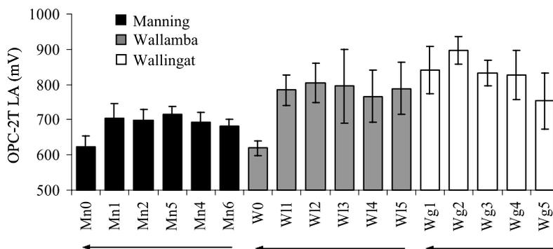
**Figure 9.** Light attenuation (mean  $\pm$  SE) measured in situ by the OPC-2T at each site in the Manning, Wallamba, and Wallingat rivers for all sampling months. Note that the relatively undisturbed Wallingat River has the highest light attenuation. This is likely a result of tannins in the water rather than detritus or suspended particulates. Arrows point downstream for each estuary.
