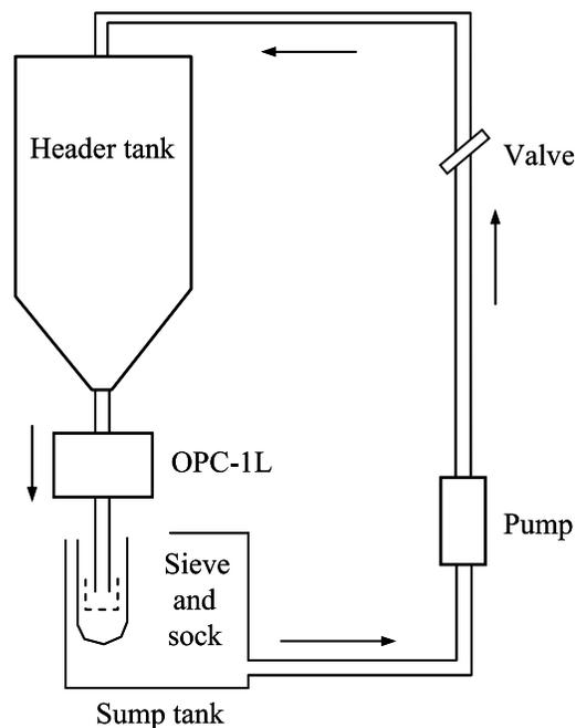
**Figure 3.** Schematic diagram of the OPC-1L circulation system. The sump and header tanks are polyethylene, and all tubing is PVC with a diameter of 1.9 cm. Arrows indicate the direction of flow.
